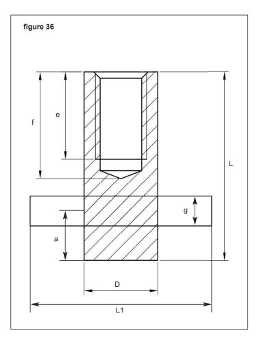
Machined from solid rod and offering a heavy wall construction, in either a zinc plated finish or stainless steel grade 304. This socket offers higher fixing capacities than its equivalent thread diameter standard fixing socket. Whilst the crossbar does not increase the fixing capacity of the Solid Rod Fixing Socket it offers improved anchorage in cracked or honeycombed concrete. The minimum design strength for surrounding concrete should be 30 N/mm<sup>2</sup>.
