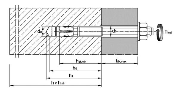
Table B2: Minimum thickness of concrete member, minimum spacings, edge distances
