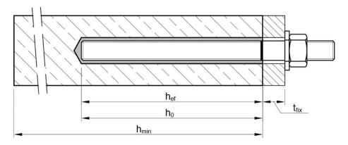
$t_{fix}$  = thickness of fixture
