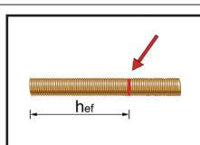
6. The position of the embedment depth shall be marked on the threaded rod. Push the threaded rod into the anchor hole while turning slightly to ensure positive distribution of the adhesive until the embedment depth is reached. The anchor shall be free of dirt, grease, oil or other foreign material.
