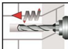
3. Holes to be drilled perpendicular to the surface of the base material by using a hard-metal tipped hammer drill bit. Drill a hole, with drilling method according to Annex C4-C45, into the base material, with nominal drill hole diameter and bore hole depth according to the size and embedment depth required by the selected anchor. In case of aborted drill hole the drill hole shall be filled with mortar.
