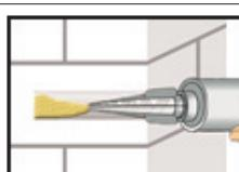
5. Starting from the bottom or back of the cleaned anchor hole, fill the hole up to min two-thirds with adhesive. Slowly withdraw the static mixing nozzle will avoid creating air pockets. Observe the gel- / working times given in Table B4.
