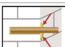
7. Be sure that the annular gap is fully filled with mortar. If no excess mortar is visible at the top of the hole, the application has to be renewed.
