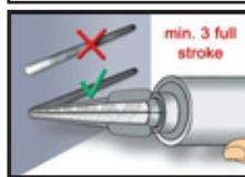
1. Remove the cap and attach the supplied static-mixing nozzle to the cartridge and load the cartridge into the correct dispensing tool. In case of a foil tube cartridge, cut off the clip before use. For every working interruption longer than the recommended working time (Table B4) as well as for new cartridges, a new static-mixer shall be used.
