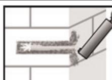
4. Blow out from the bottom of the bore hole two times. Attach the brush to a drilling machine or a battery screwdriver, brush the hole clean two times, and finally blow out the hole again two times.
