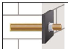
9. After full curing, the fixture can be installed with up to the max. installation torque (see parameters of brick Annex C4 to Annex C45) by using a calibrated torque wrench.
