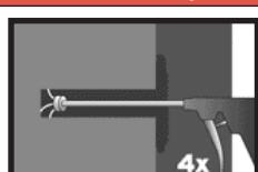
2a. Starting from the bottom or back of the bore hole, blow the hole clean with compressed air (oil free, min. 6 bar) a minimum of four times until return air stream is free of noticeable dust. If the tool does not reach the bottom of the bore hole an extension must be used.
