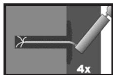
2a. Starting from the bottom or back of the bore hole, blow the hole clean by a hand pump a minimum of four times.
