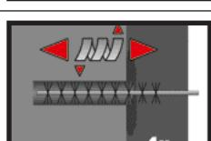
2b. Check brush (BR) diameter (table above). Brush the hole with an appropriate sized wire brush a minimum of four times in a twisting motion over the entire embedment depth of drilled hole. If the brush does not reach the bottom of the bore hole a brush extension must be used.
