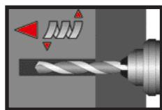
1. Drill a hole into the base material to the size and embedment depth required by the selected anchor (page 4). In cases of aborted drill holes, the drill hole must be filled with mortar.
