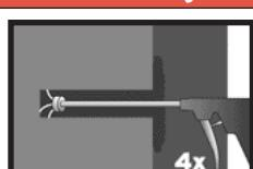
2a. Starting from the bottom or back of the bore hole, blow the hole clean with compressed air (oil free, min. 6 bar) a minimum of four times until return air stream is free of noticeable dust. If the bottom of the bore is not reached an extension must be used.
