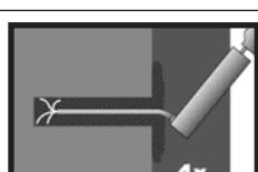
2c. Finally blow the hole clean again with a hand pump a minimum of four times from the bottom of the drilled hole.
