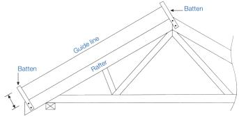
75mm + thickness of roof covering
