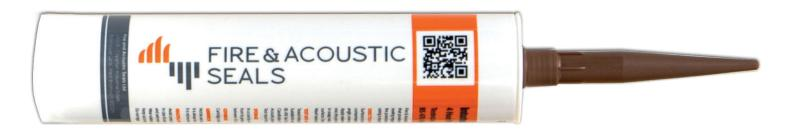
Fire & Acoustic Seals FR Intumescent and Acoustic Acrylic Sealant is a halogen free, polymer emulsion based sealant that swells when subjected to temperatures in excess of 125°C and forms a char coat that restricts the passage of smoke and fire. It is easily applied and dries to a flexible and smooth surfaced material which is readily over paintable. It has excellent adhesion to a wide range of substrates and will not harden or crack with age.
