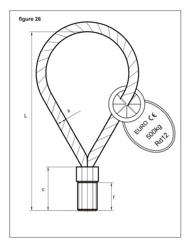
Euro Accessories Threaded Lifting Loops are suitable to be used with all sizes of threaded lifting sockets. They are economical and can be used in most applications. Threaded Lifting Loops are not suitable for turning or pitching. They can be reused, but only after inspection. Threaded Lifting Loops should only be attached to the concrete unit and used after the concrete strength has reached 20.0 N/mm².
