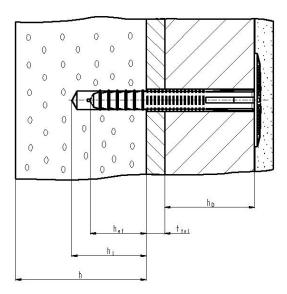
**Intended use**: anchorage of ETICS in concrete and masonry.
