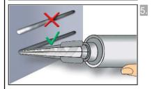
Prior to dispensing into the anchor hole, squeeze out separately a minimum of three full strokes and discard non-uniformly mixed adhesive components until the mortar shows a consistent grey colour.
