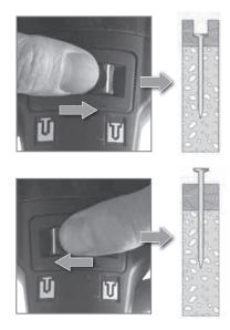
The minimum and maximum penetration is adjusted by using a button on the front of the tool.
