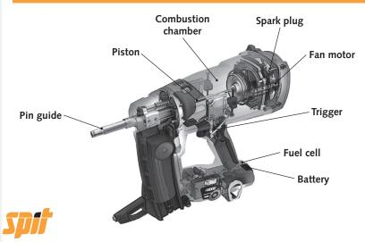
PULSA is powered by easily replaceable fuel cells. Each time the nose of the tool is depressed a metered amount of air and fuel gas mixture is injected into the combustion chamber where it is ignited by a spark when the trigger is pressed.
