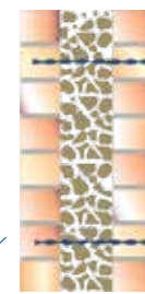
Crack-stitching (see crack stitching leaflet)
