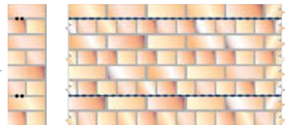
Repairing cracks near corners and openings (see crack-stitching leaflet)
