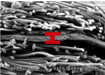
Standard multilayer Membrane: 30 microns (internally measured)
