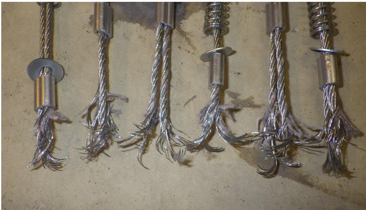
Image 9: All 6 Whipchecks after test
