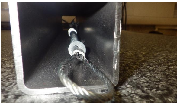
Image 2: Whipcheck inserted through box section
