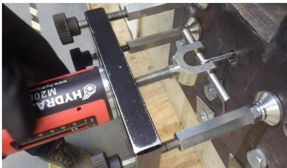
Image 4: End attached to clevis of Hydrajaws
