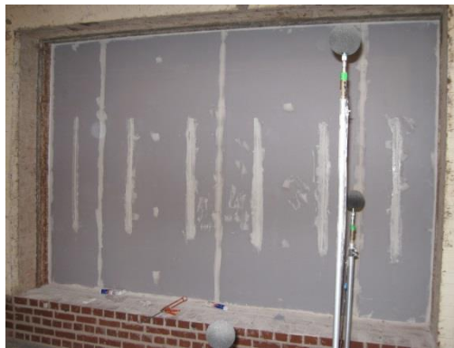
View of Partition from the Source Room
