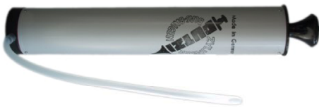
MAC - Hand pump (volume 750 ml) Drill bit diameter ( d_0 ): 10 mm to 20 mm Drill hole depth ( h_0 ): < 10 d_{nom} Only in non-cracked concrete
