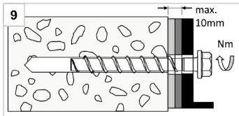
After adjustment, tighten the screw again
