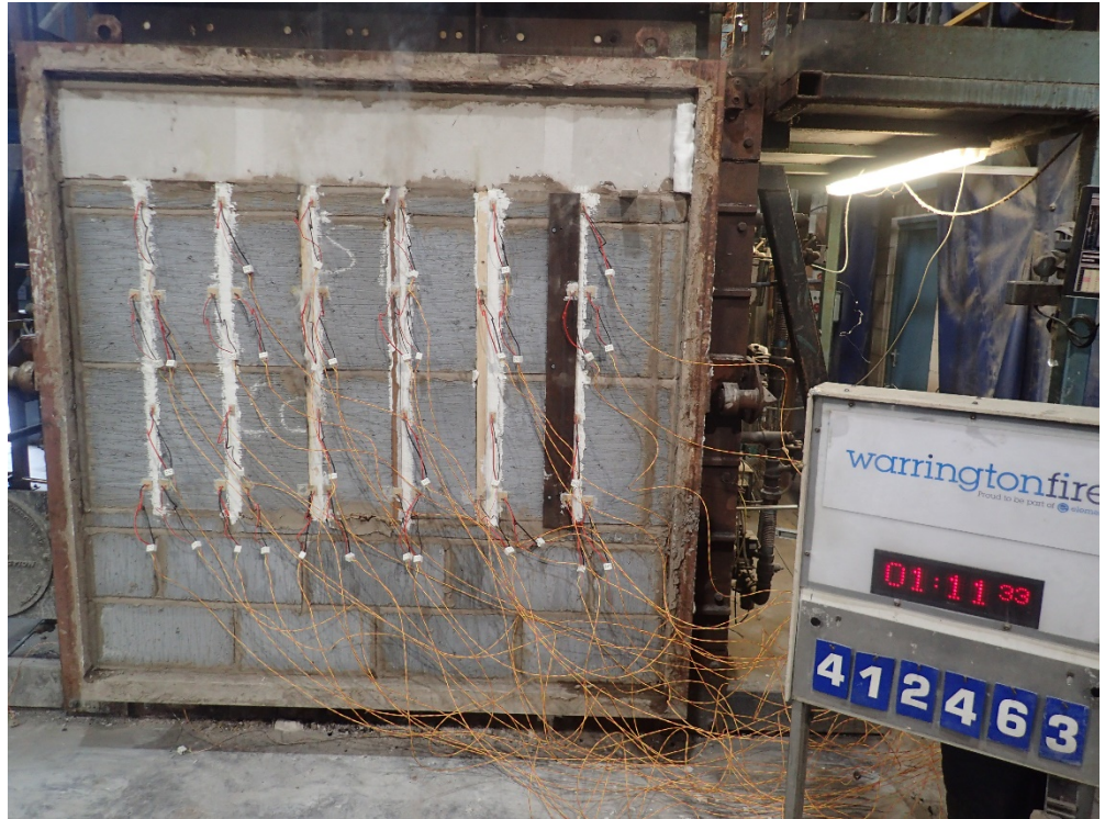
The unexposed face of the wall construction after a test duration of 71 minutes
