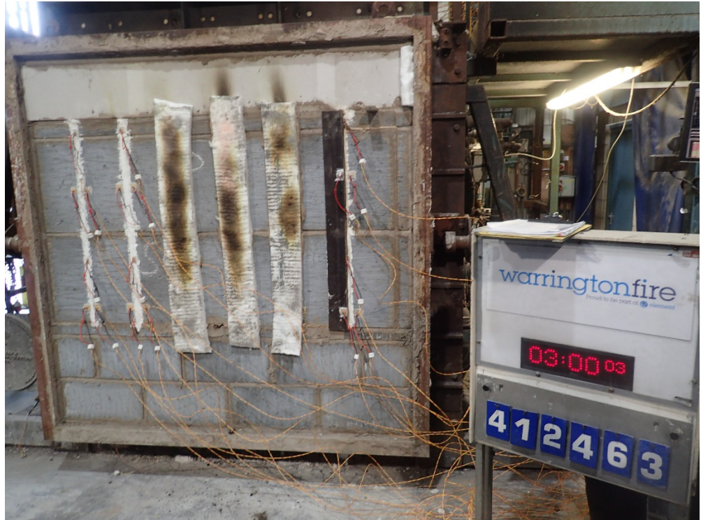
The unexposed face of the wall construction after a test duration of 180 minutes
