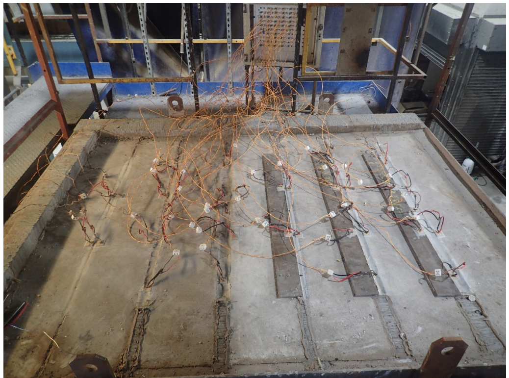
The unexposed face of the floor construction prior to testing
