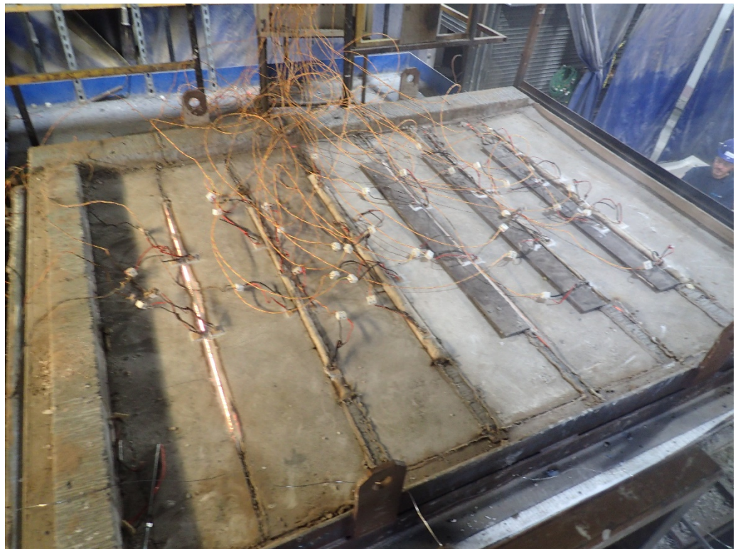
The unexposed face of the floor construction after a test duration of 180 minutes
