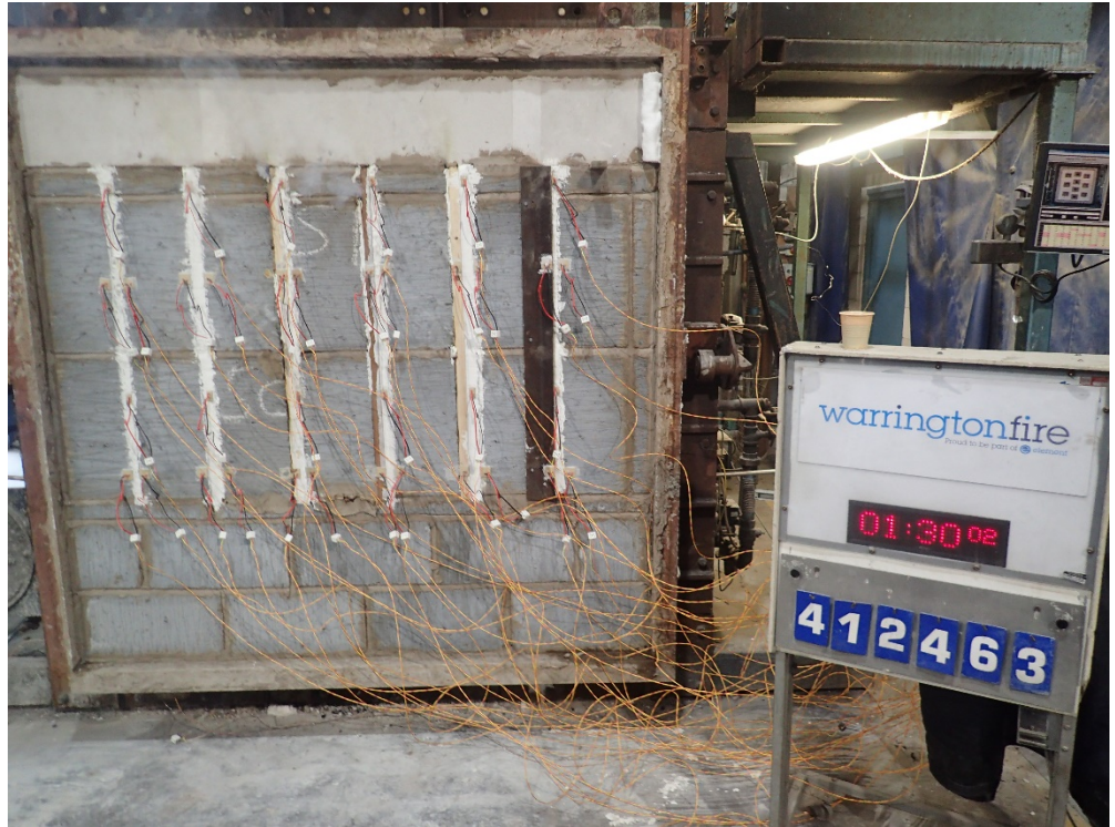
The unexposed face of the wall construction after a test duration of 90 minutes
