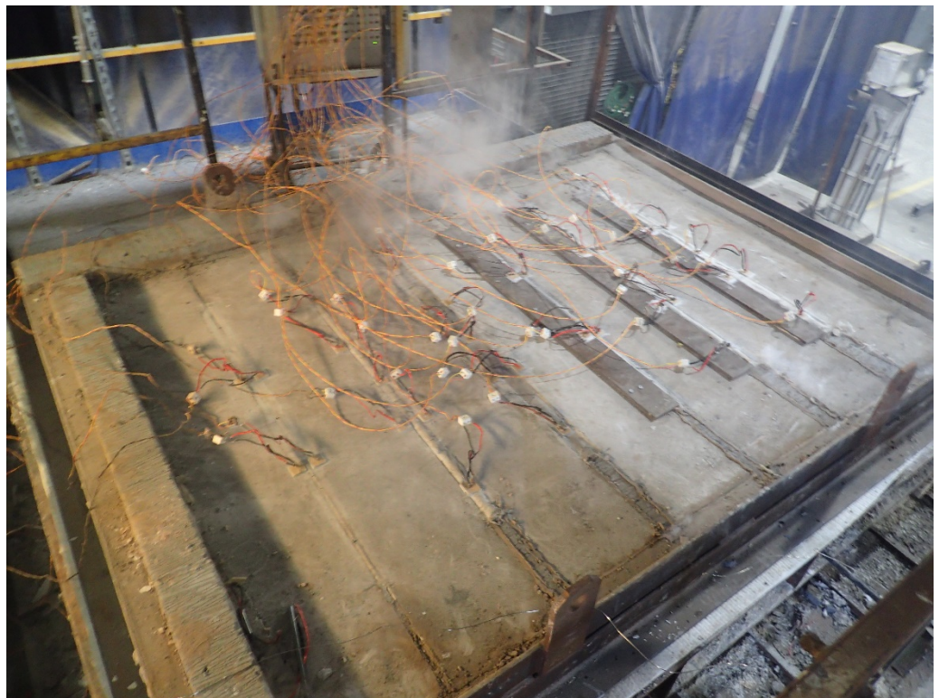
The unexposed face of the floor construction after a test duration of 30 minutes
