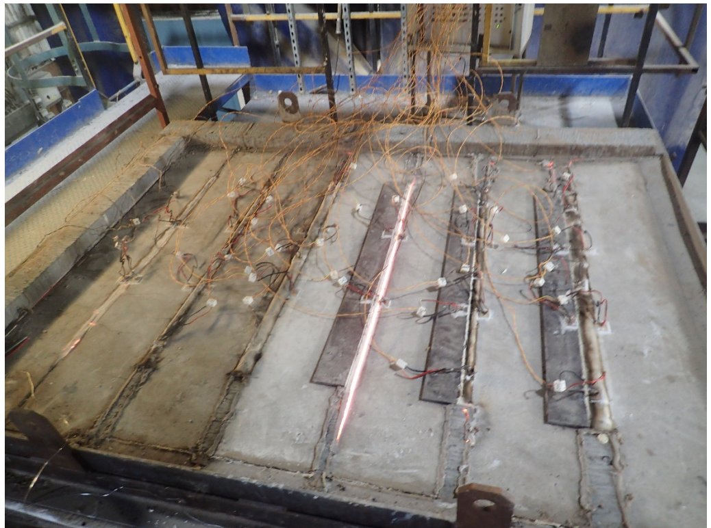
The unexposed face of the floor construction after a test duration of 240 minutes
