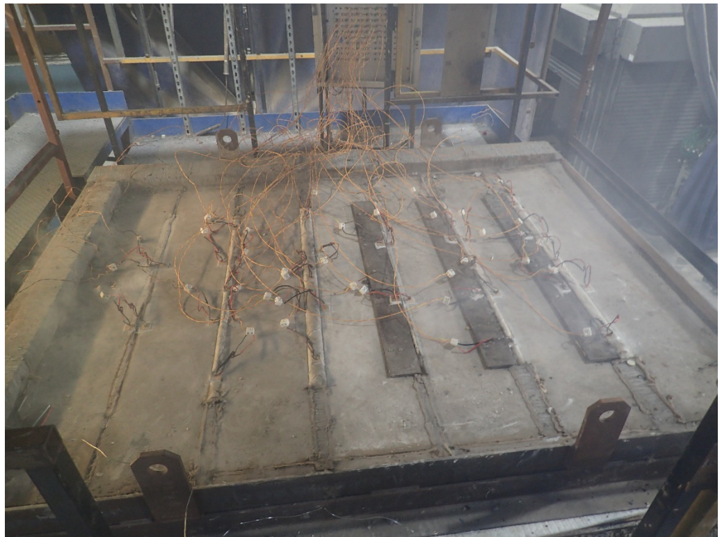
The unexposed face of the floor construction after a test duration of 90 minutes
