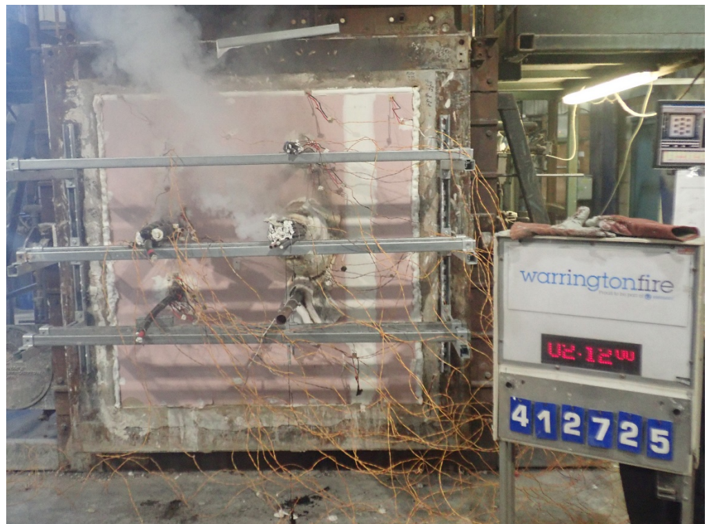
The unexposed face of the wall construction after a test duration of 132 minutes
