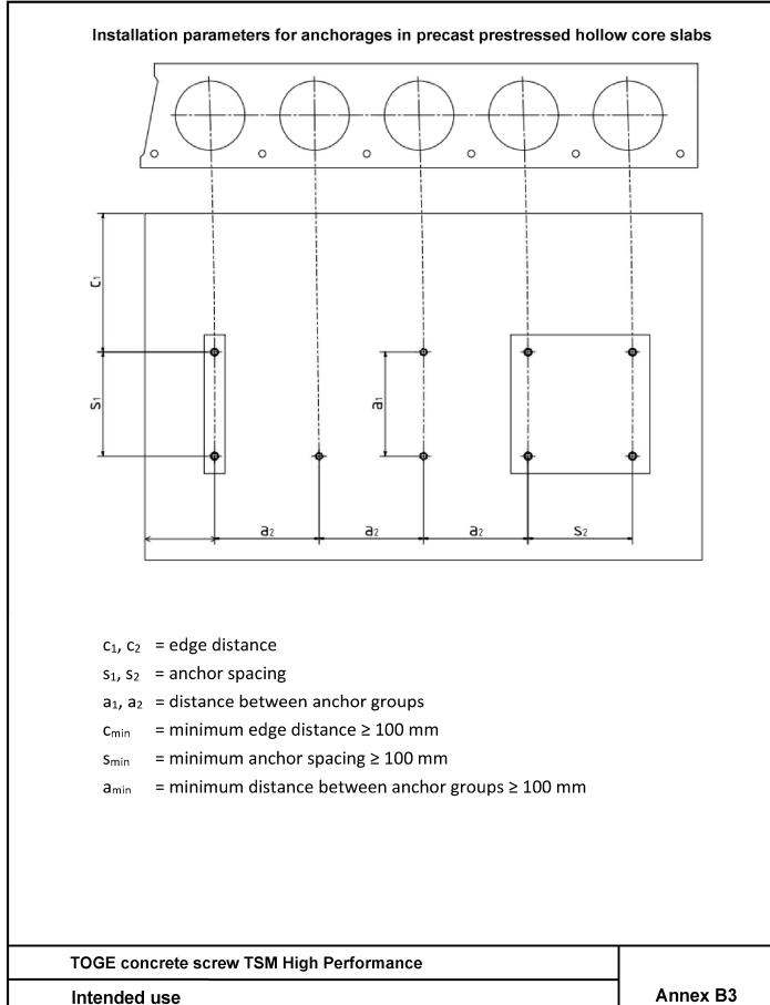
Installation parameters for anchorages in precast prestressed hollow
